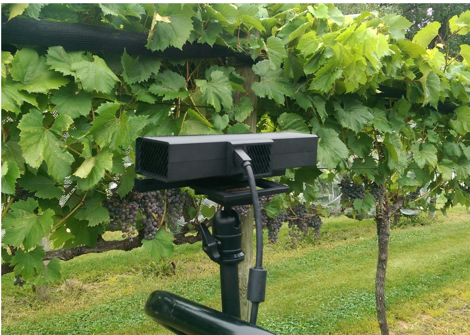
Measuring canopy density using a Kinect2 3D/LIDAR camera
