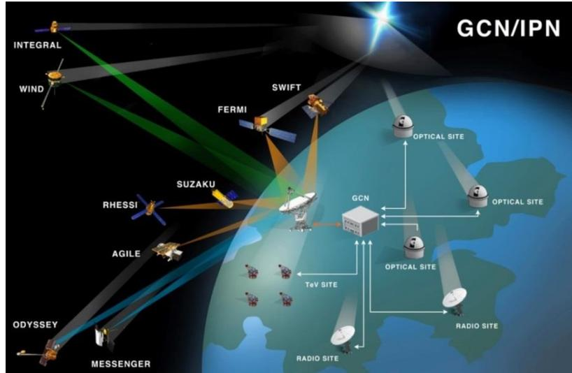
**Figure 3. The integrated GCN and spacecraft-based IPN architecture.**
