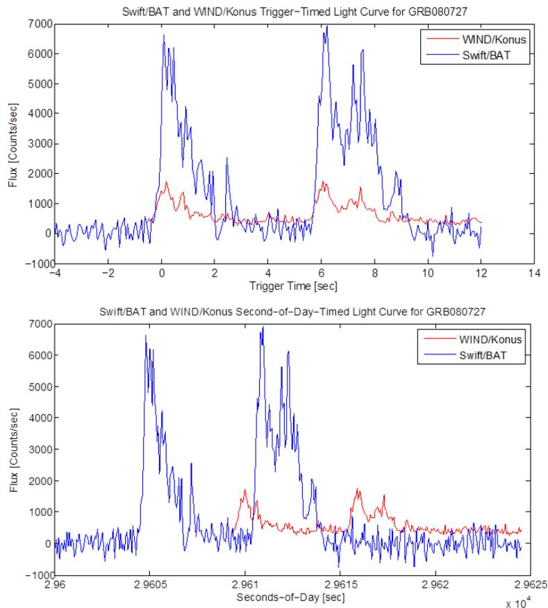
**Figure 6. Comparisons using two GRB instruments for GRB080727B, using trigger time (top panel) and second-of-day (bottom panel).**
