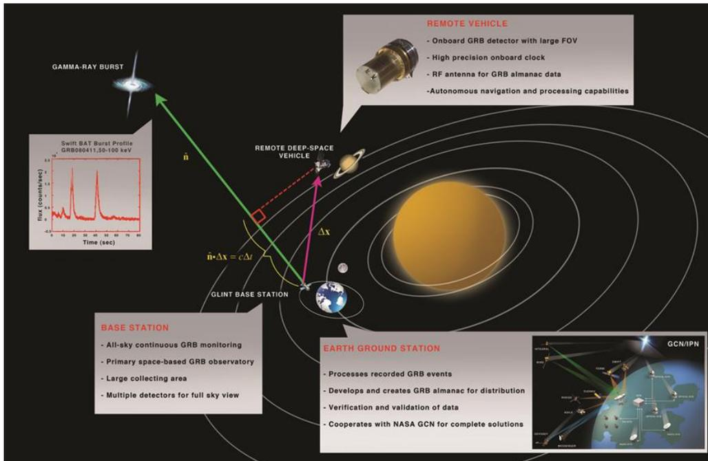
**Figure 4. The GLINT concept and architecture for spacecraft navigation.**
