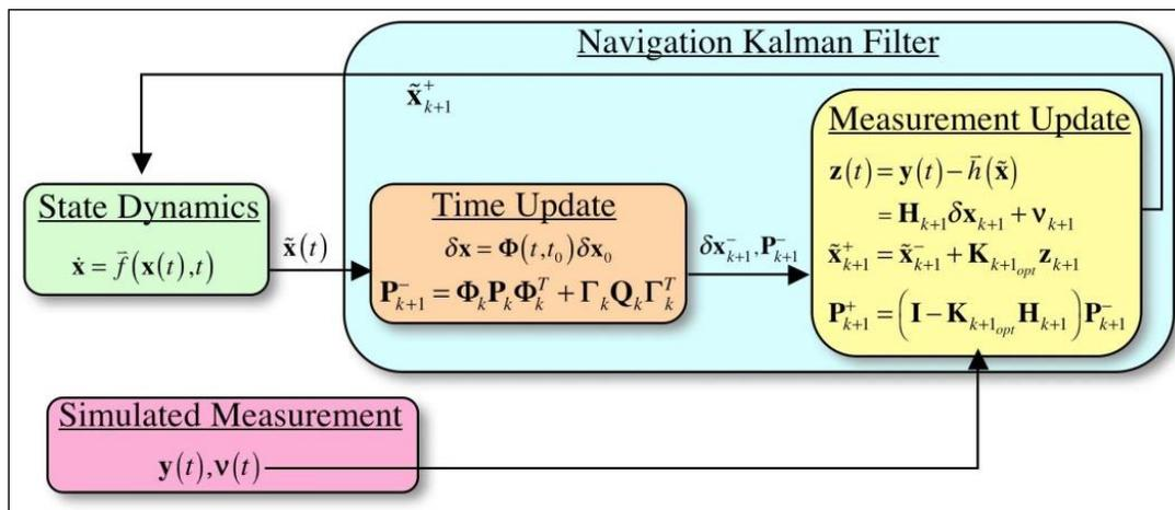
**Figure 8. Kalman filter dynamics and measurement processing data flow.**
