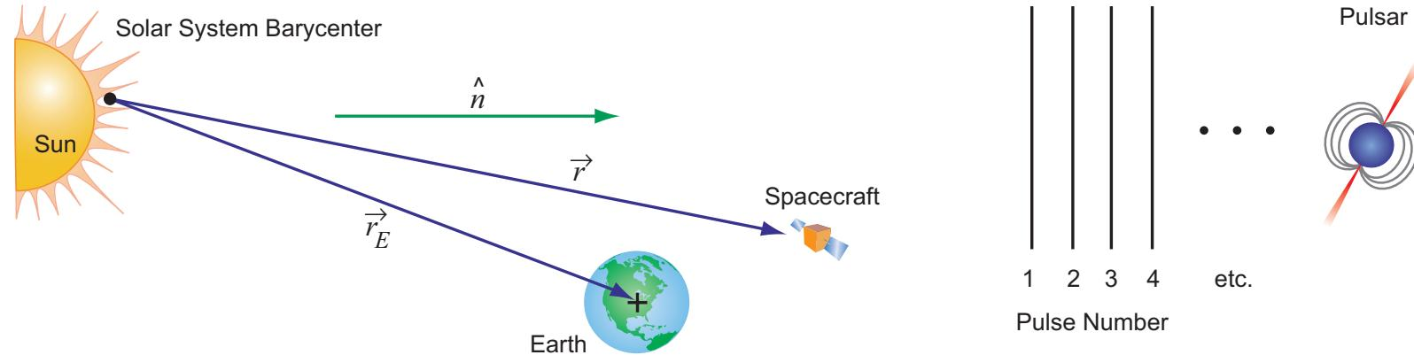
Pulsating X-ray sources, predominately rotation-powered pulsars, can be used as navigation beacons to provide position and time information for a spacecraft. This is the inverse problem to TEMPO and is a kind of natural analog to the Global Positioning System (GPS).
